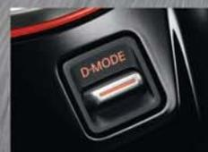
**STANDARD MODE/ ECO MODE/SPORT MODE\*\*\*.** Select ECO for enhanced fuel efficiency, Standard for the best balance between fuel efficiency and performance, or Sport for maximum thrills.
